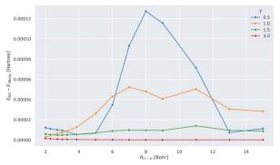
Fig. 1 Error introduced by neglecting the pure three-body contribution in the normal-ordered  $\hat{H}_{tc}$  with respect to the Hartree–Fock determinant. The absolute error is given with respect to the electronic energy obtained with the full  $\hat{H}_{tc}$  along the potential energy curve of LiH. Each curve corresponds to a tcDMRG calculation performed in the cc-pVDZ basis with a distinct value of  $\gamma$  in the correlator  $\tau = \frac{1}{a} \sum_{l'|j} r_{ij} e^{-\gamma r_{ij}}$ .
