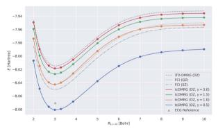
Fig. 3 LiH tcDMRG ground-state potential energy curves (cc-pVDZ (DZ) basis set, normal-ordered approximation) obtained with different values of  $\gamma$ . For comparison, imaginary-time time-dependent DMRG (iTD-DMRG) results in the cc-pVDZ basis, and FCI results obtained with the larger cc-pVQZ (QZ) and cc-pV5Z (5Z) basis sets are given. An explicitly correlated Gaussian (ECG) result<sup>227</sup> is provided as a highly accurate estimate of the exact Born–Oppenheimer energy.
