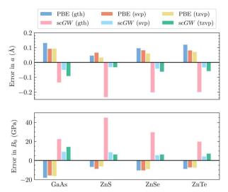
Fig. 2 Errors in (top) lattice constants a, and (bottom) bulk moduli  $B_0$  for selected materials. All compounds are calculated with GTH-DZVP-MOLOPT-SR, x2c-SVPall and x2c-TZVPall basis sets. Both AE-PBE and AE-scGW results are reported using the sfX2C1e Hamiltonian, with a  $4 \times 4 \times 4$  k-mesh sampling. Experimental values for lattice constants and bulk moduli can be found in ref. 104, 105 and 106–108 respectively.
