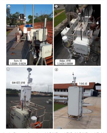
Fig. 2 Pictures of monitors, (a) RAMPs at UFHB, (b) RAMPs at UG, (c) colocation of BAM-1022 and RAMPs at UFHB, (d) Teledyne T-640 at UG.
