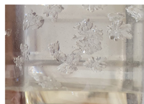
Fig. 2 A collection of N 2 O 5 crystal clusters. Note that the clusters are usually up to 1–1.5 cm across.
