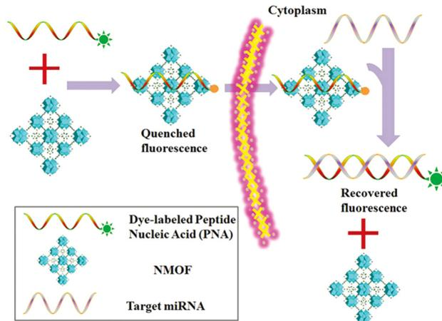
Fig. 16 Schematic diagram of the PANMOF sensing mechanism.<sup>102</sup> Reproduced with permission. Copyright 2015, RSC.
