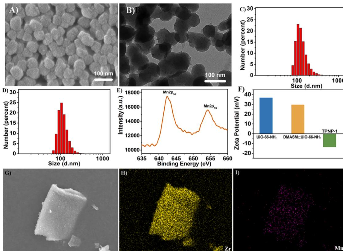
Fig. 14 (A) SEM image of TPNP-1 (scale bar = 100 nm). (B) TEM image of TPNP-1 (scale bar = 100 nm). (C) DLS data of TPNP-1. (D) DLS data of DMASM-UiO-66-NH<sub>2</sub>. (E) XPS plot of TPNP-1. (F) Zeta potential diagram for UiO-66-NH<sub>2</sub>, DMASM-UiO-66-NH<sub>2</sub> and TPNP-1. (G–I) SEM-mapping image of TPNP-1.<sup>97</sup> Reproduced with permission. Copyright 2021, Elsevier.
