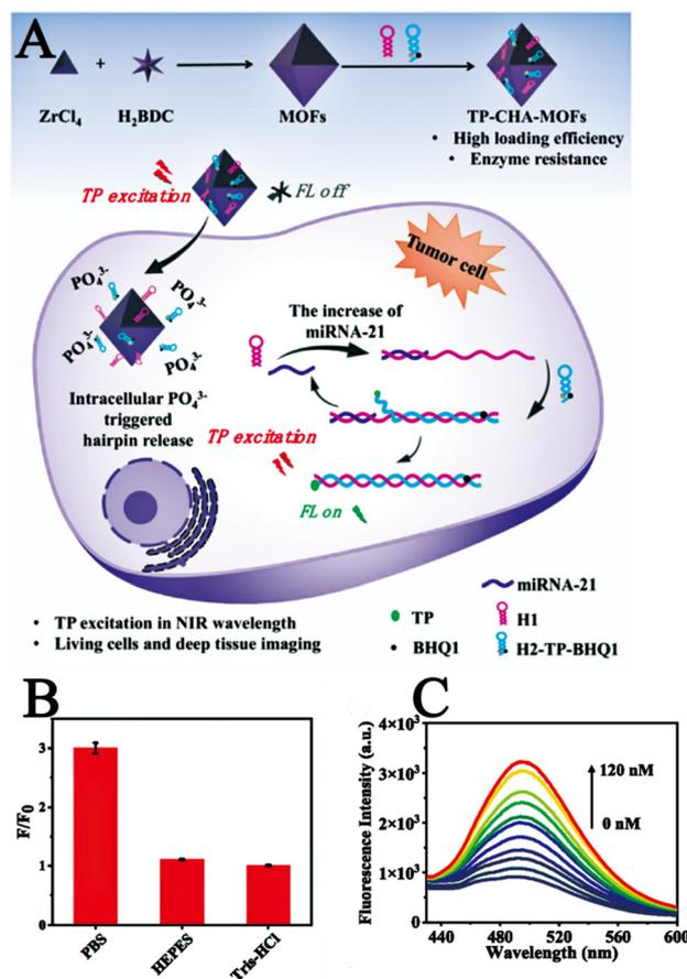
Fig. 18 (A) Schematic diagram of the imaging process of TP-CHA-UiO-66 in living cells. (B)  $F/F_0$  for TP-CHA-MOFs incubated with miRNA in DPBS, HEPES, or Tris-HCl buffer. (C) Fluorescence spectra of various concentrations of miRNA (0–120 nM).<sup>105</sup> Reproduced with permission. Copyright 2022, Elsevier.
