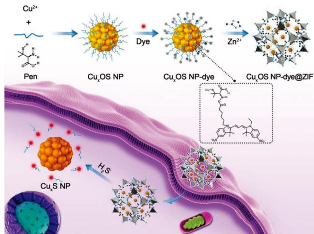
Fig. 12  $\text{Cu}_x\text{OS}@ZIF-8$ . Schematic diagram of detecting  $\text{H}_2\text{S}$  in cells using a nanosensor.<sup>83</sup> Reproduced with permission. Copyright 2020, Wiley.
