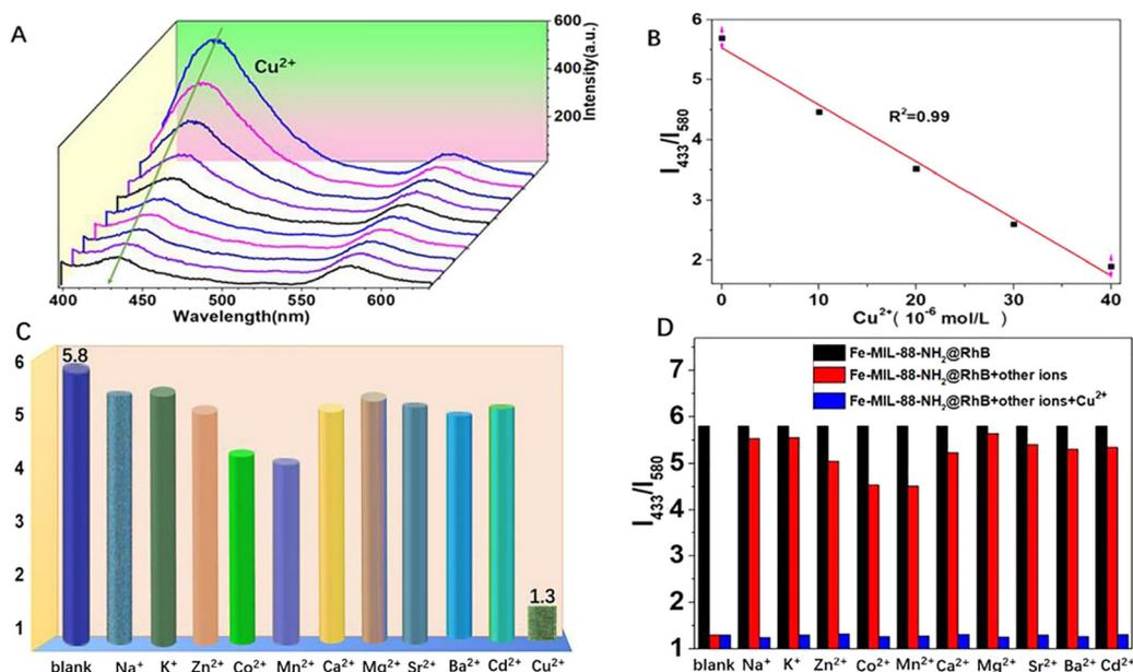
Fig. 9 (A) Luminescence spectra of Fe-MIL-88NH<sub>2</sub>@RhB at different Cu<sup>2+</sup> concentrations in aqueous solution. (B) Standard curve of Cu<sup>2+</sup> concentration. (C) Fluorescence intensity response of Fe-MIL-88NH<sub>2</sub>@RhB to other metal ions. (D) Interference test of Fe-MIL-88NH<sub>2</sub>@RhB against other metal ions.<sup>73</sup> Reproduced with permission. Copyright 2021, Elsevier.
