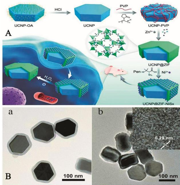
Fig. 6 (A) Schematic diagram of the UCNP@MOF-NiS<sub>x</sub> nanocomponent used to detect intracellular H<sub>2</sub>O<sub>2</sub>. (B) (a) a TEM image of the UCNP@ZIF nanostructure; (b) a TEM image of the UCNP@MOF-NiS<sub>x</sub> nanocomponent and the inset shows a high-resolution TEM image of NiS<sub>x</sub> in the nanocomponent.<sup>61</sup> Reproduced with permission. Copyright 2019, *Journal of the American Chemical Society*.
