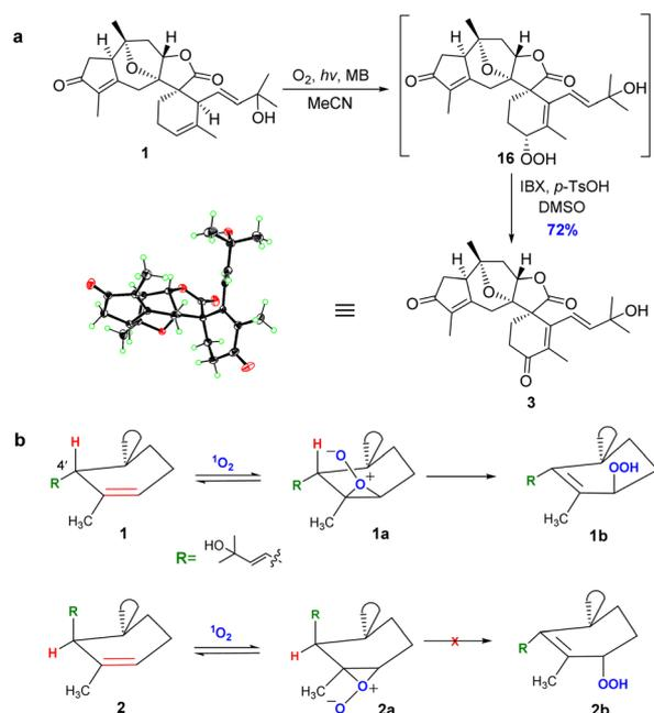
Scheme 5 (a) Synthesis of orientanoid C (**3**). MB = methylene blue; IBX = 2-iodoxybenzoic acid; *p*-TsOH = *p*-toluenesulfonic acid; DMSO = dimethylsulfoxide. (b) Stereoselectivity for the singlet oxygen ene reaction of compounds **1** and **2**.
