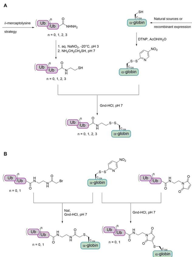
Fig. 12 Preparation of ubiquitinated  $\alpha$ -globin variants with different cysteine-linkages. (A) The Ub was linked to the  $\alpha$ -globin via a reducible disulfide bond. (B) The Ub was linked to the  $\alpha$ -globin via a stable thioether bond.
