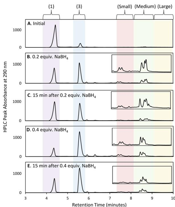
Fig. 9 Chromatograms for synthesis of 4 *via* dose-wise addition of  $\text{NaBH}_4$  with regional analysis zones identified and highlighted. Sample taken before the addition of  $\text{NaBH}_4$  (A), immediately following first addition of 0.2 equiv.  $\text{NaBH}_4$  (B), and 15 min after  $\text{NaBH}_4$  (C), additional 0.2 equiv.  $\text{NaBH}_4$  (0.4 equiv. cumulative total) (D) and 15 min delay (E).
