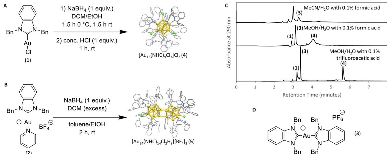
Fig. 1 (A) Conditions for the synthesis of **4** (B) conditions used for the synthesis of **5**, (C) chromatogram for the optimization of HPLC methods showing the effective separation of major species in synthesis of **4**. (D) Structure of byproduct (**3**).
