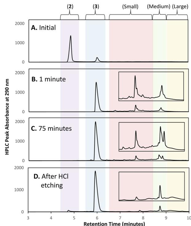
Fig. 2 Chromatograms of the synthesis of **4** taken at four critical points in the reaction with regional analysis zones identified and highlighted. Sample taken before the addition of NaBH<sub>4</sub> (A), immediately following addition of NaBH<sub>4</sub> (B), after 75 minutes of reaction time (C), and after HCl etching (D).
