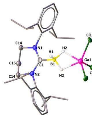
Fig. 1 The molecular structure of **1**. Hydrogen atoms (except the hydrogens attached with boron atom) are omitted for clarity. Selected bond distances (Å), bond angles (deg), and torsion angle (deg): C1–N1 1.337(3), C1–N2 1.337(3), B1–C1 1.596(6), B1–H1 1.10(4), B1–H2 1.08(3), Ga1···B1 2.280(5), Ga1–H2 1.83(3), Ga–Cl1 2.1755(8); N1–C1–N2 119.3(3), N2–C1–B1 120.29(16), N1–C1–B1 120.29(16), C1–B1–H2 112.3(17), C1–B1–H1 112(2).
