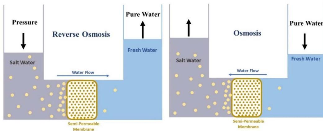
Fig. 1 Schematic of osmosis and reverse osmosis technology.
