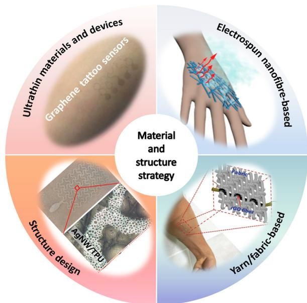
**Fig. 2** Four approaches to material and structure strategy for breathable skin-mountable electronics. Reproduced with permission from ref. 50–53. Copyright 2020 Elsevier; 2021, 2020 American Chemical Society; 2018, 2019 Wiley-VCH.
