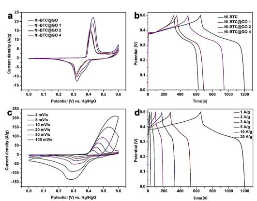
Fig. 8 (a) CV curves of Ni-BTC and Ni-BTC@GO composites at 2 mV s $^{-1}$ , (b) GCD curves of Ni-BTC and Ni-BTC@GO composites at 1 A g $^{-1}$ , (c) CV curves of Ni-BTC@GO 2 at 2 $^{-1}$ 0 mV s $^{-1}$ , and (d) GCD curves of Ni-BTC@GO 2 at 1 $^{-1}$ 20 A g $^{-1}$ 1. Reproduced from ref. 151 with permission from American Chemical Society, Copyright 2023.
