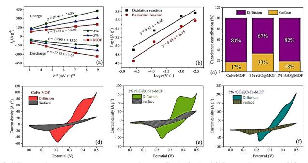
Fig. 18 (a) The curves of the peak current *versus* the square root of sweep rate (Randles–Sevcik plot). (b) The plots of  $\log i$  *versus*  $\log \nu$ . (c) Capacitance contribution for three electrodes, the capacitive contribution of CV curves at 10 mV s<sup>-1</sup> for (d) CoFe-MOF, (e) 3% rGO@CoFe-MOF, and (f) 5% rGO@CoFe-MOF. Reproduced from ref. 173 with permission from Elsevier Ltd, Copyright 2023.
