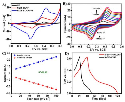
Fig. 14 CV curves of bare NF, N-ZIF-67/NF, and N-ZIF-67·rGO/NF in 2 M KOH with a scan rate of 50 mV s<sup>-1</sup> (A), CV curves of NZIF-67·rGO/NF in 2 M KOH at different scan rates (B), anodic and cathodic peak currents for N-ZIF-67·rGO/NF as a function of scan rate (C), and GCD curves of N-ZIF-67/NF and N-ZIF-67·rGO/NF in 2 M KOH at a current density of 20 mA (D). Reproduced from ref. 164 with permission from American Chemical Society, Copyright 2021.
