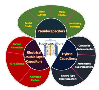
Fig. 2 Classification of supercapacitors.
