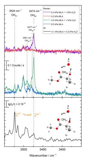
Fig. 2 Experimental Raman (top) and IR spectra (bottom) for the MLA monohydrate, showing by isotope substitution that the two OH stretching modes are coupled and that the higher-wavenumber transition OH<sub>b1</sub> is dominated by water stretching motion. See text for details.
