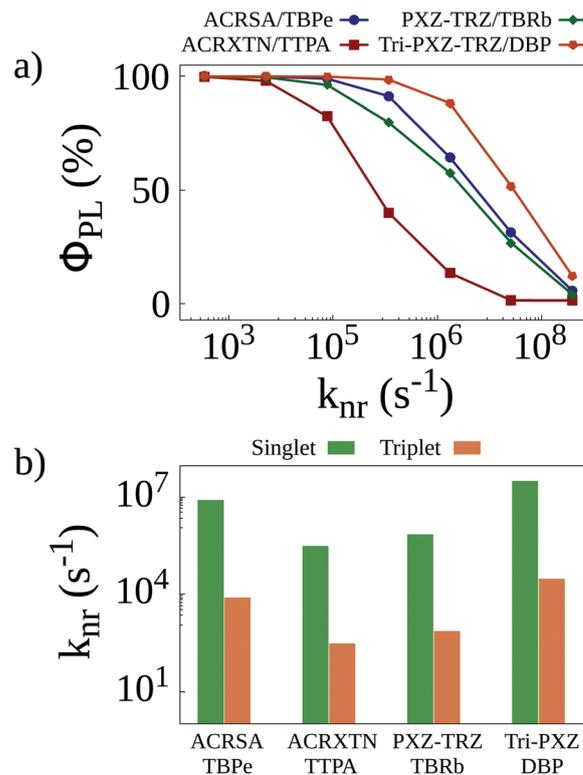
**Fig. 3** (a) Photoluminescence quantum yields as a function of the non-radiative decay rate for singlet excitons calculated for simulations with initially only singlet excitons. (b) Non-radiative decay rates that better reproduce experimentally obtained quantum yields<sup>8</sup> as a function of the energy of the emission peak of the four TADF/emitter pairs.
