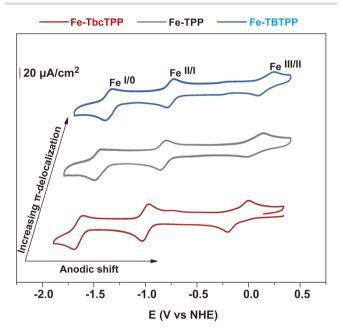
Fig. 2 Cyclic voltammetry of 0.25 mM Fe-Por dissolved in DMF containing 0.1 M TBAPF $_6$  as the supporting electrolyte, carried out at a scan rate of 100 mV s $^{-1}$ . Fe-TbcTPP (red), Fe-TPP (gray), and Fe-TBTPP (blue).
