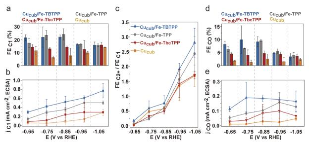
Fig. 5 (a) FE<sub>C</sub>, and (b) partial current density for the  $C_1$  products  $(j_{C_1})$  normalized by ECSA, (c) FE ratio of  $C_{2+}$  to  $C_1$  products, (d) FEs and (e) partial current density for CO ( $j_{CO}$ ) normalized by ECSA of Cu<sub>cub</sub>/Fe-TBTPP, Cu<sub>cub</sub>/Fe-TPP, Cu<sub>cub</sub>/Fe-TbcTPP and Cu<sub>cub</sub> at different potentials. The reported values are an average of three independent experiments with error bars indicating the standard deviations.
