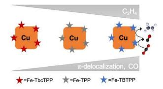
Fig. 8 Schematic representation of the proposed mechanism for  $C_2H_4$  promotion in  $Cu_{cub}/Fe-Por$  tandem catalysts. The C–C coupling enhancement and  $C_2H_4$  promotion correlate with the Fe-Por selectivity and conversion rate for CO.
