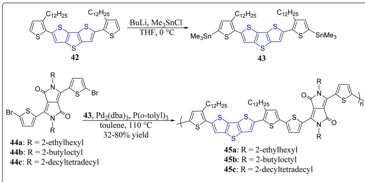
Scheme 6 Synthesis of the DTT-DPP containing conducting polymers.
