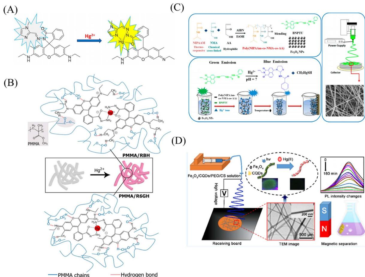
Fig. 11 Preparation and sensing mechanism of mercury ions sensor by physical doping (A) reprinted with permission from ref. 107. Copyright 2017, Elsevier. (B) Reprinted with permission from ref. 108. Copyright 2021, Elsevier. (C) Reprinted with permission from ref. 109. Copyright 2017, MDPI. (D) Reprinted with permission from ref. 110. Copyright 2018, American Chemical Society.
