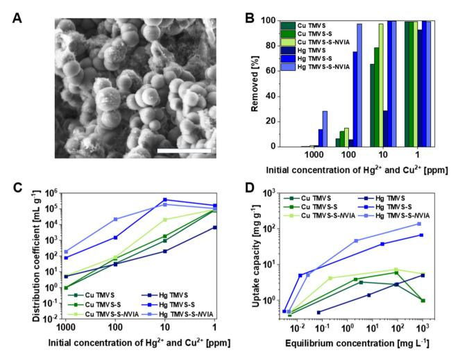
Fig. 2 (A) SEM image of TMVS-S-NVIA particles. Scalebar is 5 µm. (B) Removed copper ions (green) and mercury ions (blue) from aqueous solution by TMVS-S and TMVS-S-NVIA particles in %. Calculated distribution coefficients (C) and uptake capacities (D) of TMVS-S particles and TMVS-S-NVIA particles, respectively. Uptake capacities plotted against initial ion concentration can be found in the ESI.†
