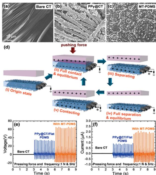
Fig. 4 SEM of textile-based electrodes (pure and chemically modified) (a)–(c); schematic view of the operation of the TENG (d) and (e) and (f)  $V_{OC}$  and  $I_{SC}$  curves of the resulting devices. Reprinted with permission from ref. 52. Copyright 2019 American Chemical Society.
