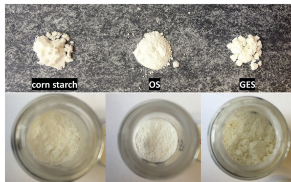
Fig. 4 Unmodified corn starch (left), OS (center), and GES (right) shown as either a pile of powder (top images) or the top-down view of a vial full of material (bottom images) showing the significant differences in physical properties.
