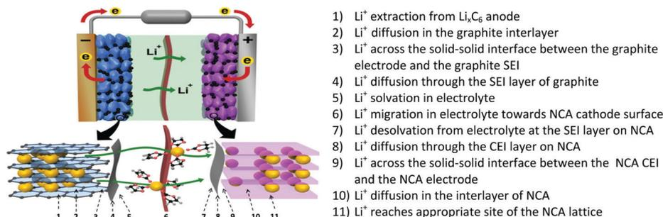
**Fig. 2** Complete overview of lithium transport pathway in a graphite||LiNi<sub>0.80</sub>Co<sub>0.15</sub>Al<sub>0.05</sub>O<sub>2</sub> full cell. The identity of the rate-limiting step may change with temperature, depending on the active material properties and electrolyte composition. Reprinted with permission from ref. 15. Copyright 2017 American Chemical Society.
