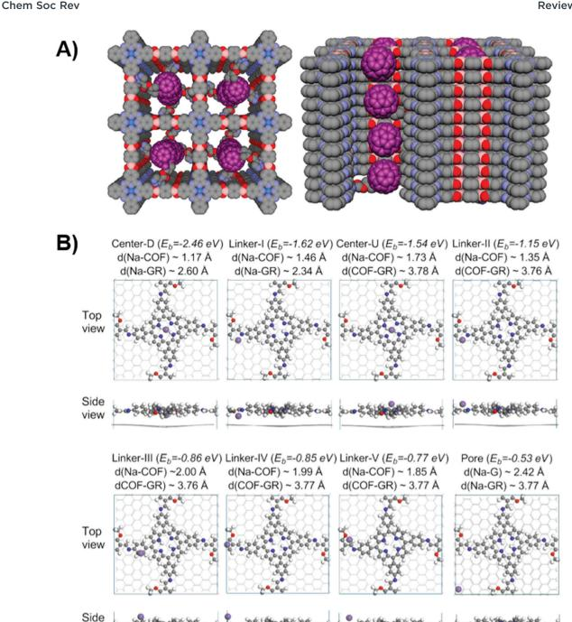
Fig. 2 (A) Top and side views of donor-acceptor COF with C<sub>60</sub> (purple) integrated on the channel walls. Reproduced with permission from ref. 100. Copyright 2014, American Chemical Society. (B) Different Na dopants calculated preferential positions with reference to graphene substrate and COF. Purple, white, grey, blue, and red balls refer to Na, H, C, N, and O atoms respectively. Reproduced with permission from ref. 108. Copyright 2020, American Chemical Society.
