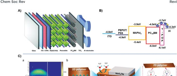
Fig. 8 (A) Device configuration of CON/PEDOT: PSS HTL incorporated PSC. Reproduced with permission from ref. 87. Copyright 2018, Royal Society of Chemistry. (B) Device incorporating T-POP as a secondary ETL. Reproduced with permission from ref. 90. Copyright 2020, Elsevier. (C) GIWAXS plot with device configuration. Reproduced with permission from ref. 92. Copyright 2021, American Chemical Society.
