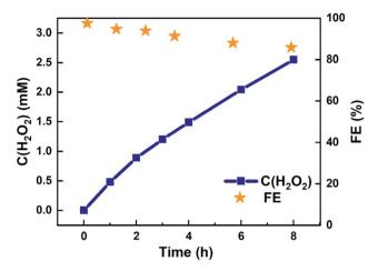
Fig. 3  $H_2O_2$  accumulation using 4: 1 (Ti,Mn)O<sub>x</sub>-coated FTO electrode operated in the dark. Cumulative  $H_2O_2$  concentration and the respective cumulative FE vs. time. The electrode area was 1.2 cm², and the applied potential was +1.31 V vs. Ag/AgCl (equivalent to an overpotential of 150 mV) in a 20 mL 0.5 M pH = 7.0 PB solution.
