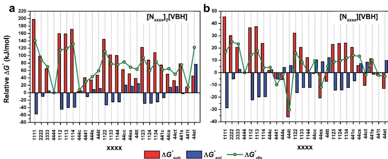
Fig. 6 Free energies of sublimation ( $\Delta G_{\text{sub}}^*$ ), solvation ( $\Delta G_{\text{sol}}^*$ ) in MeCN, and dissolution ( $\Delta G_{\text{dis}}^*$ ) in MeCN of the  $[N_{xxxx}]_y[\text{VBH}]$  active materials in the (a) +4 (where  $y = 2$ ) and (b) +5 (where  $y = 1$ ) states relative to the free energies of  $[N_{4444}]_2[\text{VBH}]$  and  $[N_{4444}][\text{VBH}]$ , respectively.
