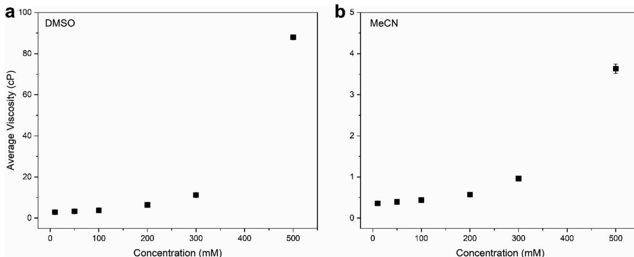
Fig. 9 Viscosity measurements of  $[N_{4444}]_2[VBH]$  in (a) DMSO and (b) MeCN at 0.01 M, 0.05 M, 0.1 M, 0.2 M, and 0.5 M concentrations. All experiments were performed using a viscometer at room temperature (25 °C).
