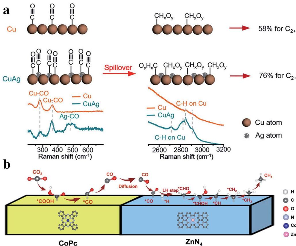
Fig. 12 (a) CO<sub>2</sub>RR mechanism for producing C<sub>2+</sub> products on Cu and CuAg catalysts. Reproduced with permission from ref. 113. Copyright (2019) American Chemical Society. (b) A proposed reaction mechanism of the CO<sub>2</sub>RR to CH<sub>4</sub> over CoPc@Zn-N-C. Reproduced with permission from ref. 116. Copyright (2020) Wiley-VCH.
