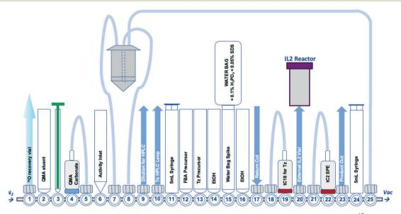
Fig. 2 A schematic representation of the GE FASTLab<sup>TM</sup> cassette developed for the automated radiosynthesis of [ $^{18}$ F]TTCO-IL2; a detailed description of the cassette setup appears in the ESI $^{\dagger}$  (Fig. S14).
