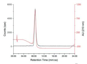
Fig. 3 Representative HPLC chromatogram showing [18F]TTCO-IL2 (grey line) co-injected with non-reactive TCO-PEG<sub>4</sub>-IL2 (red line).
