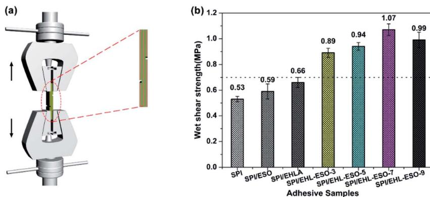
Fig. 7 Wet shear strength of plywood bonded by different soy protein-based adhesives: (a) the schematic diagram of test instrument, (b) the results of wet shear strength.
