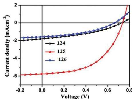
Fig. 22 Current–voltage characteristics of optimized photovoltaic cells based on **124**: PC<sub>61</sub>BM, **125**: PC<sub>61</sub>BM and **126**: PC<sub>61</sub>BM under illumination of AM 1.5, 100 mW cm<sup>-2</sup> white light. Reproduced with permission of Elsevier.<sup>74</sup>
