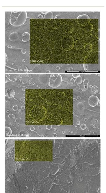
Fig. 4 SEHI images generated from the component analysis of PR382 mapping CO bonding (indicating ether bridge distributions). With the stronger emission intensity showing greater CO bonding. SEHI images are overlaid with grayscale standard SE images (integral over all energy ranges) of PR382.
