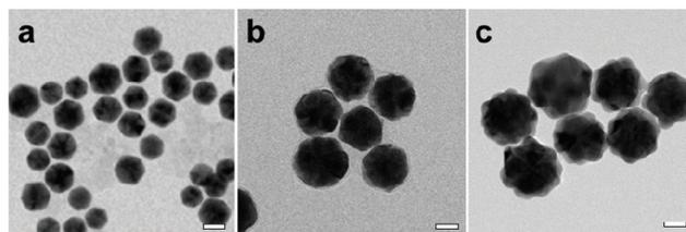
Fig. 1 TEM images of Au (a) Ih, (b) s-NS, and (c) l-NS. The bars represent 20 nm.
