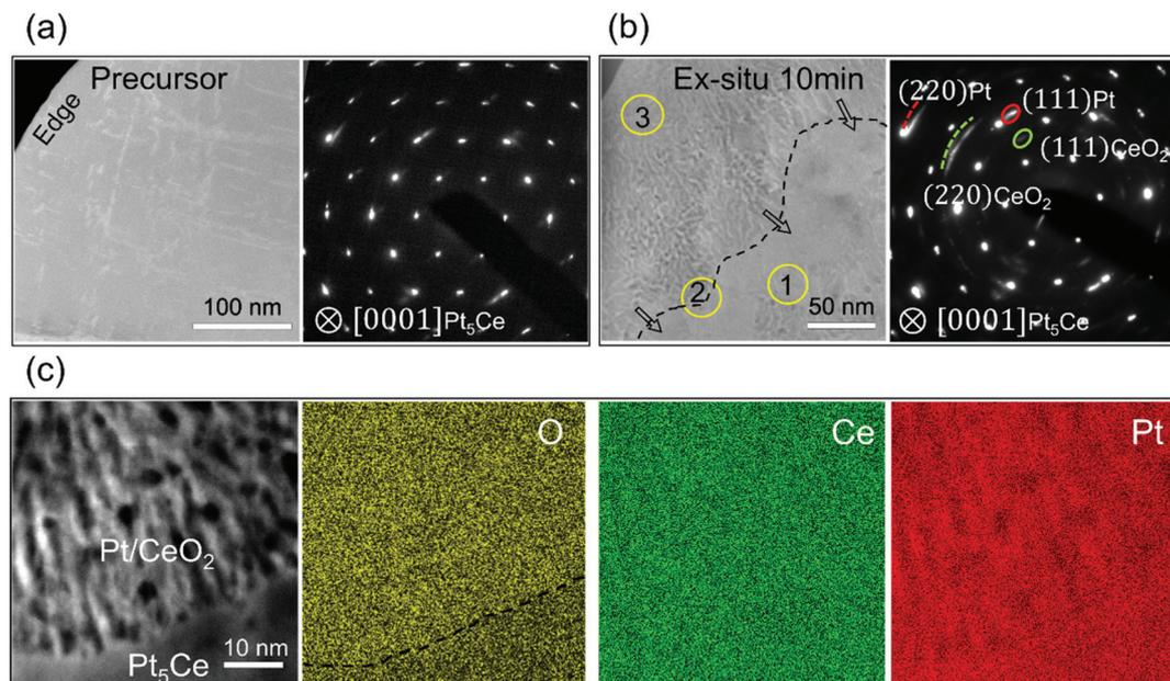
**Fig. 3** Characterization of nano-phase separation in  $\text{Pt}_5\text{Ce}$  alloy. HAADF-STEM images and corresponding SAED patterns along the  $[0001]$   $\text{Pt}_5\text{Ce}$  zone axis of (a)  $\text{Pt}_5\text{Ce}$  alloy precursor and (b) the firstly-FIB-thinned specimen *ex situ* annealed at  $400^\circ\text{C}$  for 10 min. (c) HAADF-STEM image of the interface area containing the alloy precursor and separated phases, and corresponding elemental maps of O, Ce and Pt.
