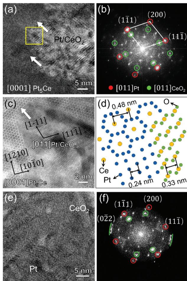
**Fig. 5** (a) HRTEM image with  $[0001]Pt_5Ce$  zone axis and (b) corresponding FFT of the middle separation stage (region 2 in Fig. 3(b)) showing the interface area between  $Pt_5Ce$  alloy and  $Pt/CeO_2$  composites. (c) HAADF-STEM image of the boxed area in (a), and (d) atomic structure model of each phase in the interface area. (e) HRTEM image along the  $[0001]Pt_5Ce$  zone axis and (f) corresponding FFT of the late separation stage (region 3).
