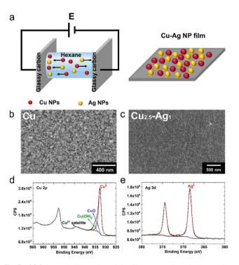
Fig. 3 (a) Schematic illustration of the film preparation via electrophoresis. The arrows indicate the moving direction of NPs under applied potential. (b and c) SEM images of the anode Cu (b) and Cu<sub>2.5</sub>-Ag<sub>1</sub> (c) NPs film prepared at 100 V for 60 min. (d and e) Cu 2p (d) and Ag 3d (e) XPS spectra of a Cu<sub>2.5</sub>-Aq<sub>1</sub> NPs film prepared by electrophoresis at 100 V for 60 min.
