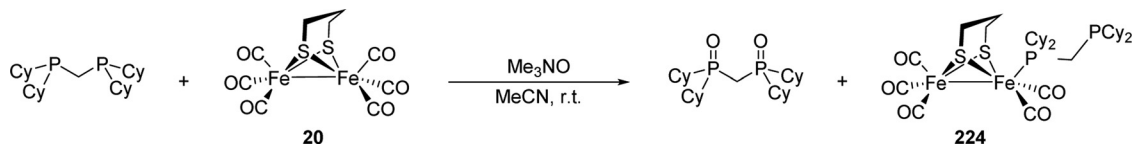
Fig. 66 Reaction of dcmp with complex 20 in the presence of \text{Me}_3\text{NO} .
