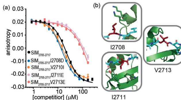
Fig. 3 FA competition data and structural analysis for SIM<sub>2705-2717</sub> and variant sequences; (a) competition FA (50 mM Tris, 150 mM NaCl, 25 nM tracer, 100 nM SUMO); (b) SIM<sub>2705-2717</sub>/SUMO (PDB ID: 2LAS) variant residues highlighted in red showing I2708 proximity to SUMO K45 and K46 residues, I2711 proximity to SUMO residues Y21 and K37 and V2713 pointing towards solvent.
