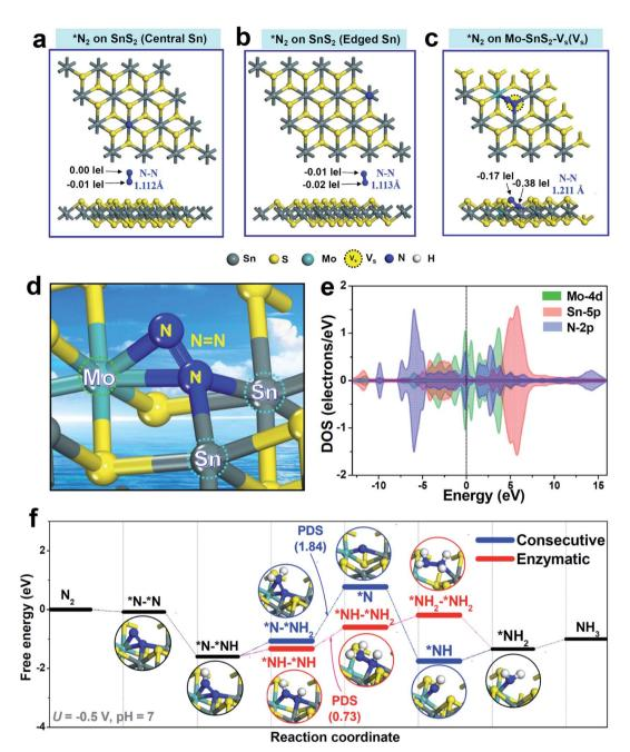
Fig. 4 (a–c) Optimized structures of  $N_2$  adsorption on (a)  $SnS_2$  (central Sn site), (b)  $SnS_2$  (edge Sn site) and (c)  $Mo-SnS_2-V_s$  ( $V_s$  site). (d) Enlarged view of the  $N_2$  adsorption mode on a  $V_s$  site of  $Mo-SnS_2-V_s$  (Mo-Sn-Sn trimer). (e) PDOS of the Mo-Sn-Sn trimer after  $N_2$  adsorption. (f) Free energy diagrams of NRR consecutive/enzymatic reaction pathways over the Mo-Sn-Sn trimer at U=-0.5 V, PM=7.
