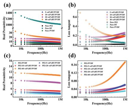
Frequency dependences of dielectric permittivity and loss tangent for (a and b) single layer and (c and d) bilayer composites.
