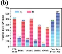
Fig. 4 (a) Weibull distribution plots and (b) characteristic breakdown strengths of the single layer and bilayer composites with different  $BaTiO_3$  loading fractions.
