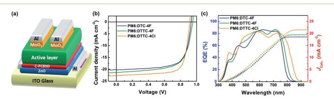
Fig. 4 (a) Illustration of the inverted OSC; (b) J-V characteristics under simulated AM 1.5 G irradiation (100 mW cm<sup>-2</sup>) and (c) EQE spectra with integrated  $J_{Calc.}$  curves.
