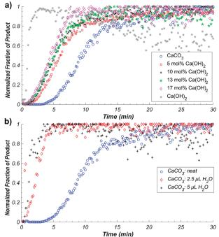
Fig. 4 (a) Monitoring the relative rates of formation of 1 from CaCO $_3$  (blue) and Ca(OH) $_2$  (grey), as well as various mixtures. (b) The addition of small volumes of water to the synthesis of 1 from CaCO $_3$ , results in a significant increase in reaction rate as observed by *in situ* Raman spectroscopy. In each case the total weight of solid reactants was approximately 180 mg.
