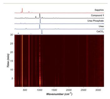
Fig. 2 (Bottom) In situ Raman spectra of the neat milling reaction between  $CaCO_3$ , urea, and urea phosphate. Brighter colour denotes higher intensity. (Top) Raman spectra of reactants (blue), the product (black), and background from the sapphire milling jar (red) with individual spectra of reactants and product above the 2D plot.
