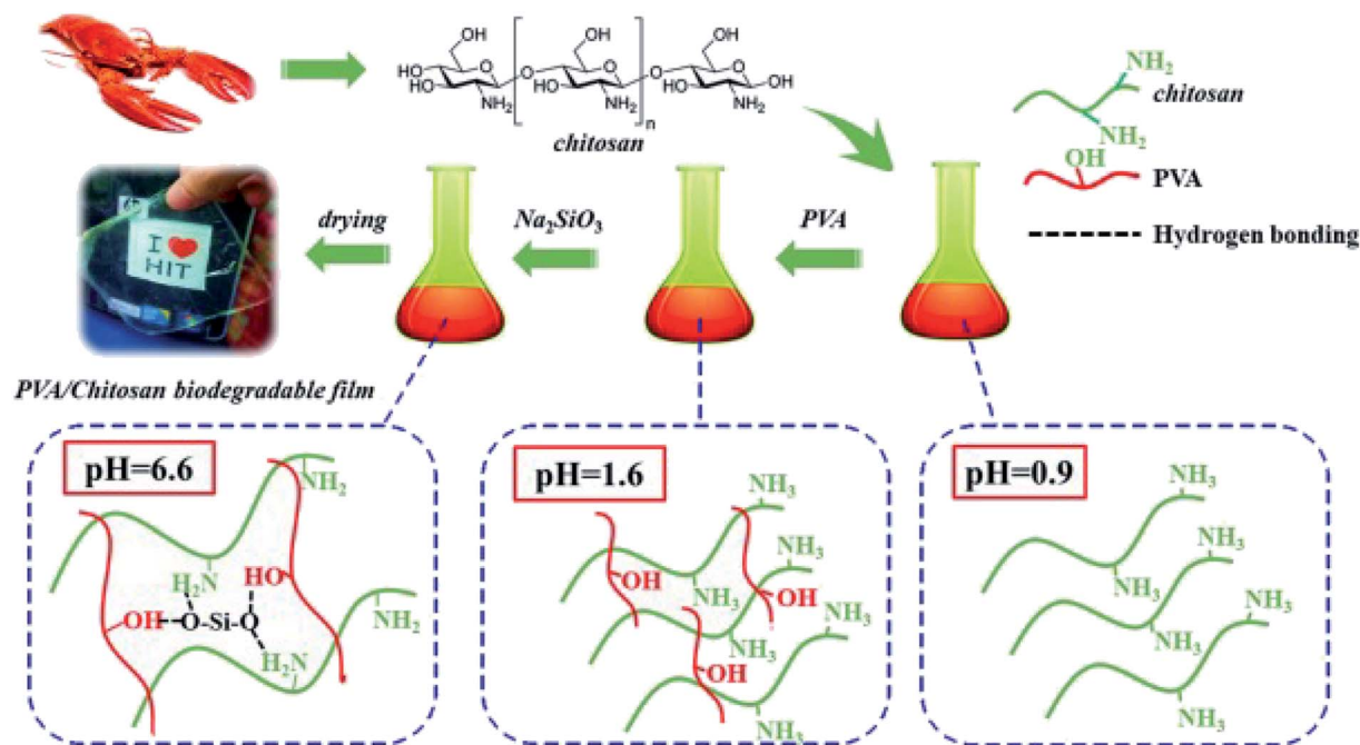
Fig. 8 \text{SiO}_2 in situ enhanced the PVA/CS biodegradable films by hydrolysis of sodium metasilicate. Reproduced with permission from ref. 64 Copyright© 2018 Elsevier.
