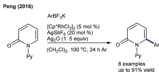
Scheme 7 Arylation of pyridones using aryl trifluoroborates.
