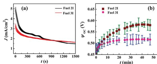
Fig. 4 (a) Chronoamperometric current density ( $J$ ) versus time ( $t$ ) studies for different  $\mu$ -DropFCs with the Fuels 2I and 3I at an applied voltage of 0.1 V. (b) The corresponding open-circuit potential ( $\psi_{oc}$ ) with  $t$  for 50 min. To demonstrate long-term performance of  $\mu$ -DropFCs, the chronoamperometry test was performed for different systems.
