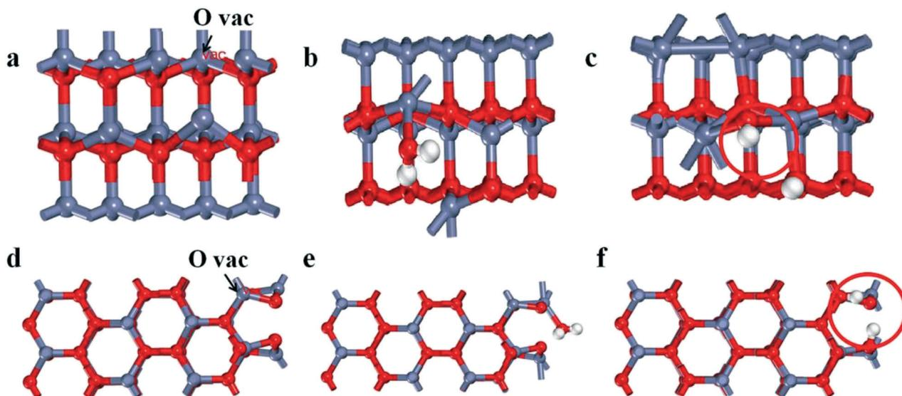
Fig. 3 Side views of the surface structures of defective ZnO (a) with O vacancies, (b) adsorption and (c) dissociation H<sub>2</sub>O on the (100) plane, side views of the surface structures of defective ZnO (d) with O vacancies and (e) adsorption and (f) dissociation H<sub>2</sub>O on the (101) plane.
