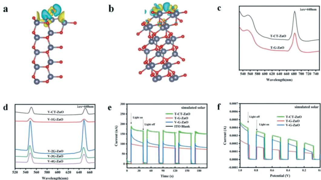
**Fig. 4** Charge difference of (a) the (100) plane and (b) the (101) plane (charge accumulation is in yellow and depletion is in blue), PL of (c) T-ZnO series samples and (d) V-ZnO series samples, (e) transient photocurrents and (f) linear sweep voltammetry.
