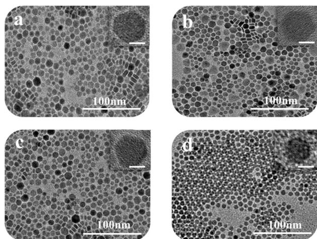
**Fig. 1** TEM images of  $\text{Cu}_{2-x}\text{S}$  nanostructures: (a)  $\text{Cu}_{1.2}\text{S}$ , (b)  $\text{Cu}_{1.4}\text{S}$ , (c)  $\text{Cu}_{1.75}\text{S}$ , (d)  $\text{Cu}_{1.94}\text{S}$  NCs. Insets: Higher magnification of individual  $\text{Cu}_{2-x}\text{S}$  NCs and the scale bar in the insets corresponds to 5 nm.
