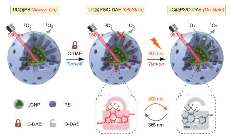
Scheme 1 Schematic illustration of the 980 nm NIR light photosensitized UC@PS/C-DAE nanoconstruct, whose  ${}^{1}O_{2}$  generation capability can be remotely switched on by 808 nm NIR light irradiation.
