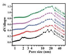
Fig. 2 (a)  $N_2$  adsorption/desorption isotherms of Ni/Al $_2$ O $_3$ -T catalyst and, (b) corresponding Barrett-Joyner-Halenda (BJH) pore-size distribution curve.
