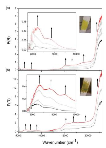
Fig. 4 Solid state Vis-NIR SEC of 1-Zn in 0.1 M  $[n-Bu_4N]PF_6/MeCN$  with arrows indicating progression of spectral bands at an applied potential of (a)  $-2.1\,V$ ; (b)  $-2.4\,V$ , with insets showing the NIR region as well as photos displaying the colour of the frameworks at respective potentials.
