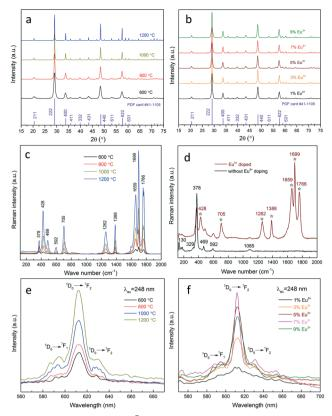
Fig. 6 XRD patterns of Eu<sup>3+</sup> doped yttria nanophosphors (a) heattreated at 600-1200 °C and (b) with a doping concentration of 1-9%, calcinated at 800 °C; Raman spectra of (c) Eu3+ doped yttria nanophosphors heat-treated at 600-1200 °C and (d) with and without Eu3+ doping; emission spectra of Eu<sup>3+</sup> doped yttria nanophosphors (e) heattreated at 600-1200 °C, 5% Eu3+ and (f) with a doping concentration of 1-9%. All spectra are excited under a UV radiation of 248 nm.
