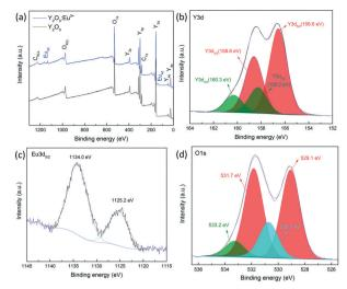
Fig. 5 (a) Full XPS spectrum of Y<sub>2</sub>O<sub>3</sub>:5%Eu<sup>3+</sup> nanoparticles annealed at 600 °C; (b) XPS spectrum of Y3d; (c) XPS spectrum of Eu3d5/2; (d) XPS spectrum of O1s.
