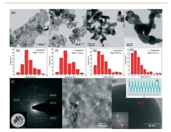
Fig. 4 TEM images of 5% Eu<sup>3+</sup> doped yttria nanophosphors with heat treatment at (a) 600 °C, (b) 800 °C, (c) 1000 °C and (d) 1200 °C; (e-h) the corresponding size distributions; (i-k) SAED pattern and HRTEM images of the 5% Eu<sup>3+</sup> doped yttria nanophosphors obtained at 1200 °C.
