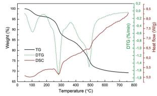
Fig. 2 Typical TG/DTG-DSC curves for the thermal decomposition of the plasma-generated Y(OH)<sub>3</sub>:5%Eu<sup>3+</sup> powders.
