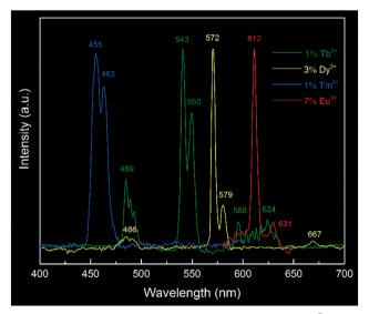
Fig. 7 Typical photoluminescence emission spectra of  ${\rm Ln}^{3+}$  doped yttria nanophosphors: 1% Tb<sup>3+</sup> doping, excited at 307 nm; 3% Dy<sup>3+</sup> doping, excited at 355 nm; 1% Tm<sup>3+</sup> doping, excited at 355 nm and 7% Eu<sup>3+</sup> doping, excited at 248 nm. All spectra were normalized at the same level. The measuring conditions were referenced to reported values in the literature.41
