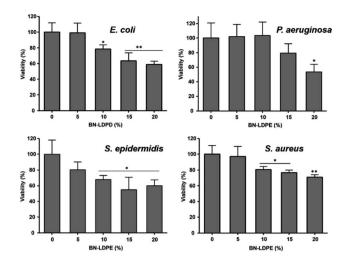
Fig. 3 Measurement of bactericidal activity extruded LDPE composites with 0–20% of BN after the 24 h of bacterial growth. Results are presented as a mean  $\pm$  standard deviation error of viability percentage of each bacterial strains in compared to control. \*P < 0.005, \*\*P < 0.001.
