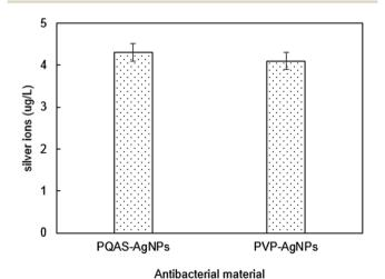
Fig. 4 The silver ion release in PQAS-AgNPs or PVP-AgNPs solution. Reaction conditions:  $[AgNPs] = 1.0 \text{ mg L}^{-1}$ , reaction time = 60 min, pH  $= 7.1, T = 25 \, ^{\circ}\text{C}.$
