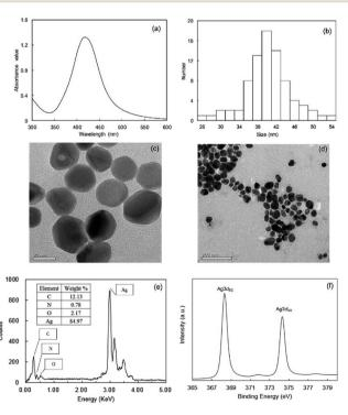
Fig. 1 Characterization of PQAS-AgNPs (a) UV-visible spectrum; (b) the size distribution; (c and d) TEM images; (e) corresponding EDS spectrum and (f) XPS spectrum.
