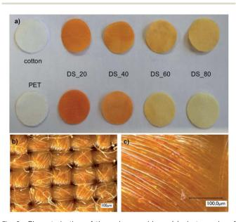
Fig. 2 Characterization of the polymer add-on: (a) photographs of textiles (cotton and PET) finished with PVAm-g-SB2 with varying DS that were stained by TNBS; (b) and (c) light microscopic pictures of PET finished with PVAm-g-SB2\_20 after TNBS staining.
