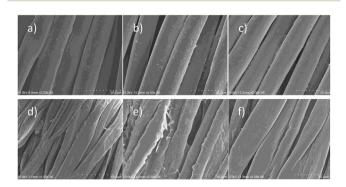
Fig. 4 SEM images of fabrics before and after finishing with PVAm-g-SB2\_20. (a) PET untreated; (b) PET directly after the finishing step; (c) PET after finishing and washing with ECE detergent; (d) cotton untreated; (e) cotton directly after the finishing step; (f) cotton after finishing and washing with ECE detergent.
